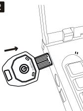
Insert the recorder into the USB port of the computer to view the PDF data report.
