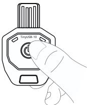
Long press for 5 seconds to start recording, the green light flashes 5 times.
